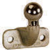
Crochet standard 2 trous Boule Ø 50 mm, traction 3,5 tonnes
